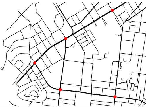
Figure 6: Topology of the real-world transportation network used in the simulations. Possible targets for an attack are marked by red disks.
